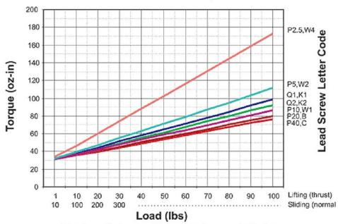
\* 1.5x torque for dynamic safety margin, 2x torque needed for startup
